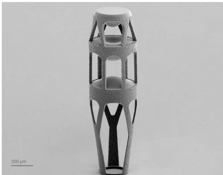
Figure 5: High-precision optics developed for a miniature endomicroscope. The stacked freeform lenses are 3D-printed by Two-Photon Grayscale Lithography. The three lenses are supported by a textured scaffold avoiding back-reflexes. All three freeform lenses have optical-grade surfaces on the top and bottom, integrating diffractive and refractive elements into one optical system and are printed in one pass. Lens design by Printoptix, manufacturing by Nanoscribe.
