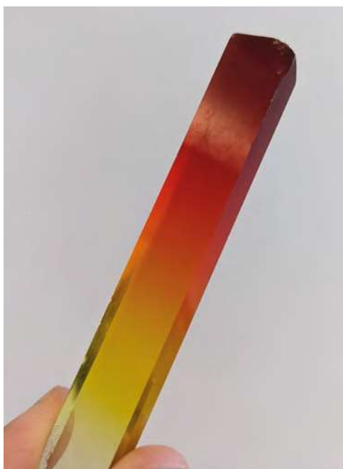
Figure 1. Image of a glass slab grown by Ekimov containing CdSe centers. The thermal treatment conducted on the glass leads to the formation of CdSe quantum dots with various sizes due to the temperature gradient, resulting in a gradient of sizes. Quantum dots at the top are large, resulting in a narrow bandgap and in absorption of almost all visible light. Quantum dots at the bottom are small, pushing their absorption spectrum to the blue resulting in enhanced optical transparency of the glass. Picture Los Alamos National Laboratory, LA-UR-23-31622.
