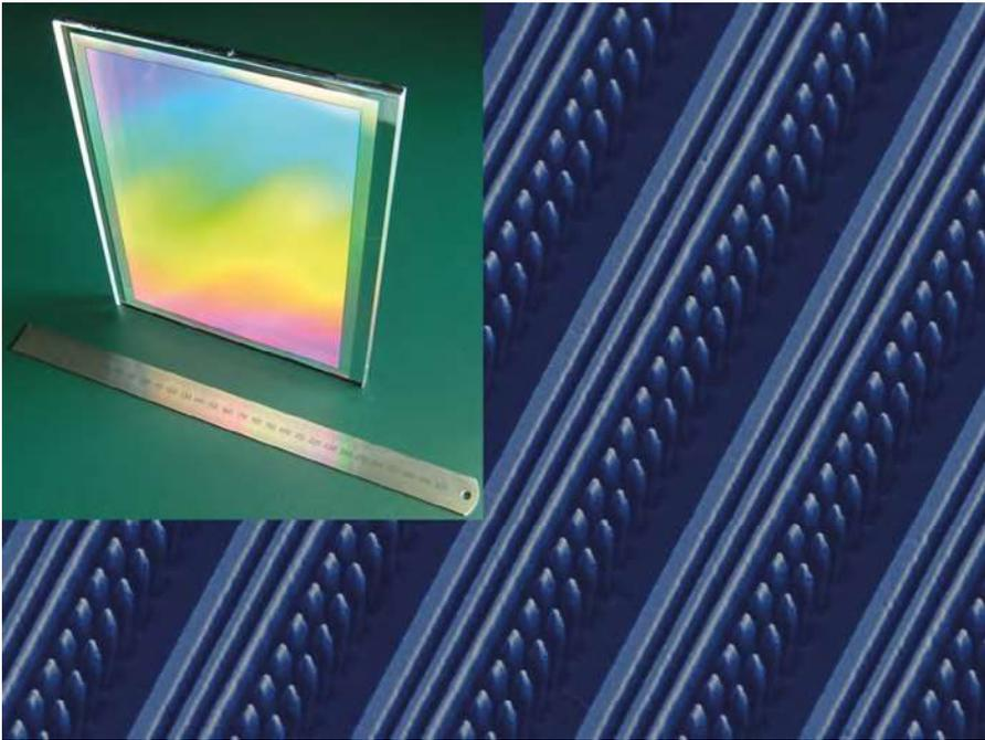
**Figure 3.** Scanning electron micrography of 20.5×15.5 cm<sup>2</sup> grating used in a spectrophotometer sent to space in 2013. The initial design was composed of pillars only for polarization insensitivity issue. Optimization has led to a combination owing to the difficulty of manufacturing high-aspect ratio pillars with large surface coverages. Courtesy Uwe Zeitner. See [6] or <http://sci.esa.int/science-e/www/object/index.cfm?fobjectid=44093>.
