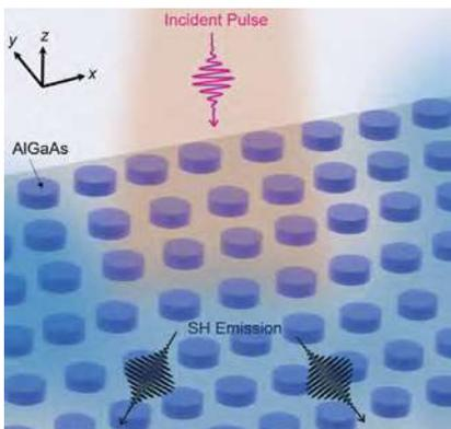
Recently, nonlinear optics at the nanoscale level has emerged as a promising branch of nanophotonics. In this work, we focus our attention on Aluminum Gallium Arsenide (AlGaAs) nanoantennas and metasurfaces for efficient and controlled second harmonic photon emission. After a brief introduction concerning the main studies in this field, we present the latest results achieved in AlGaAs platforms both in the lossless and absorption regimes.
