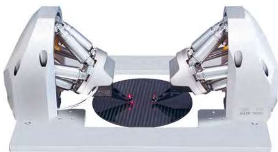
Figure 1. A double-sided test and alignment system for silicon photonics wafers based on hexapods and piezo nanopositioning stages to combine the fastest alignment speeds with the highest flexibility.
