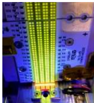
Light concentrator (LED's+Ce:YAG) pumping laser crystal (in red)
