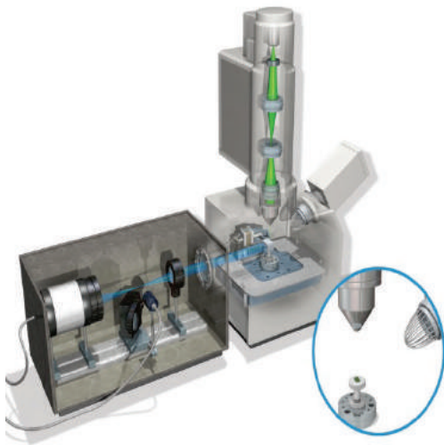
Figure 1. Cathodoluminescence microscope developed at AMOLF using a 30 keV electron beam and a parabolic mirror light collector.
