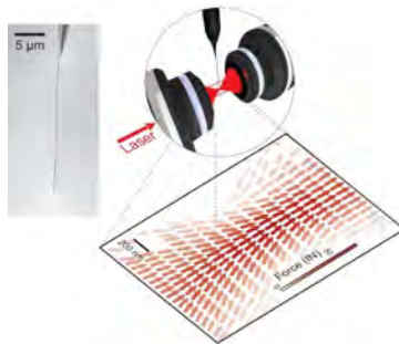
Fig. 1 Left: SEM image of a typical silicon carbide nanowire with 150 nm diameter. Right: schematics of the experiment: we cartography the optical force field exerted on the nanowire by a strongly focused laser beam.
