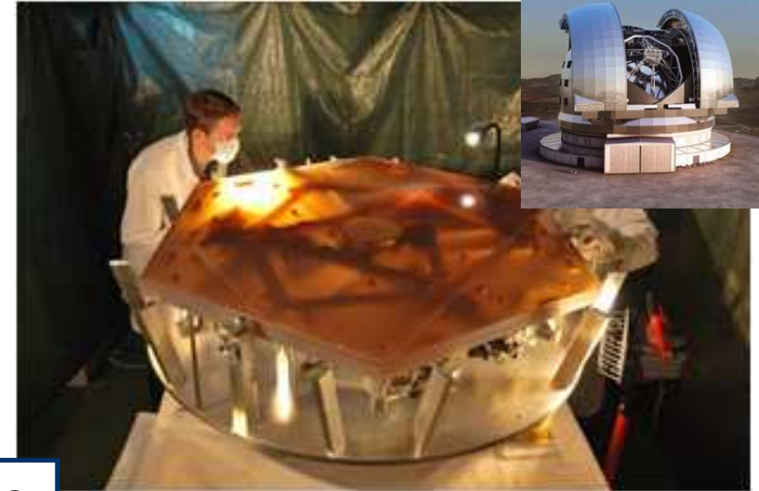
ELT M1 segments mass-production with freeform technology
