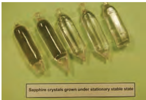
Figure 1. Sapphire crystals grown from the melt to test the quality of alumina starting powders
