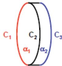
$$c_2' = [c_2/(1+\alpha_1\Delta T) + c_2/(1+\alpha_2\Delta T)]/2$$
