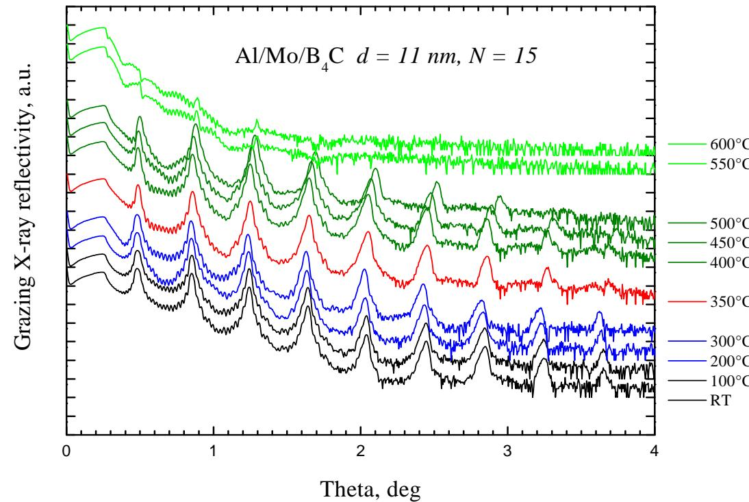
A good thermal stability of structural parameters of the multilayers upon heating to 300°C
