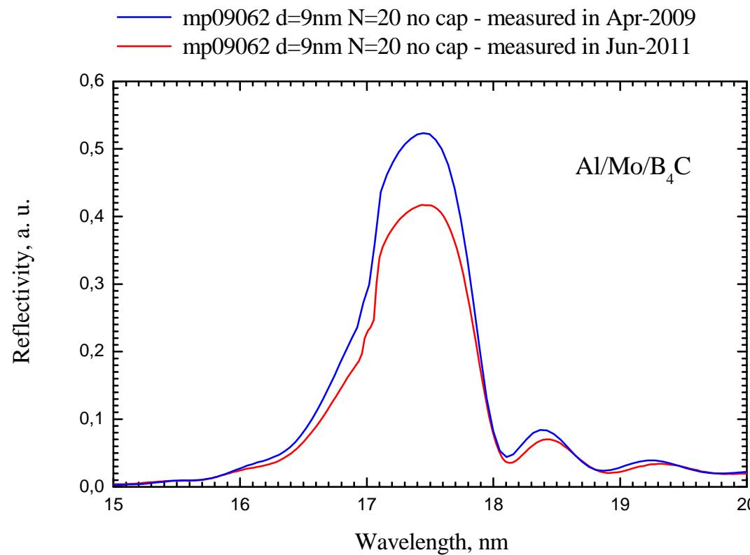
Significant reflectivity loss observed for the multilayer without protective layer stored during 2 years in air at room temperature
