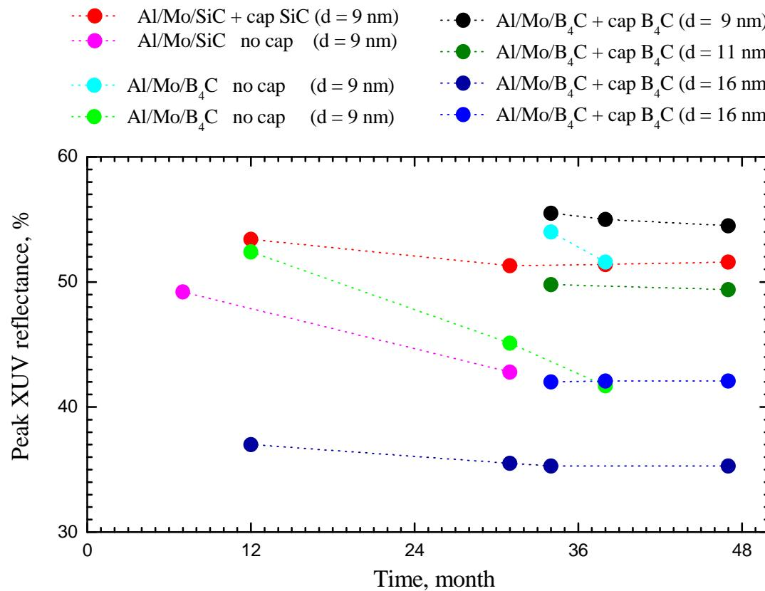
A good temporal stability of optical characteristics of the multilayers with protective layer
