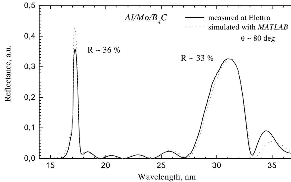
Reflectivity of bi-band  $Al/Mo/B_4C$  multilayer designed for 17 and 30 nm
