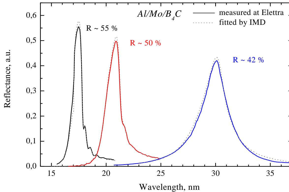
Reflectivity in the range from 15 to 35 nm of simple band Al/Mo/B<sub>4</sub>C multilayers
